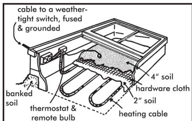
Figure 5. Layout of heating cable in a hotbed.
