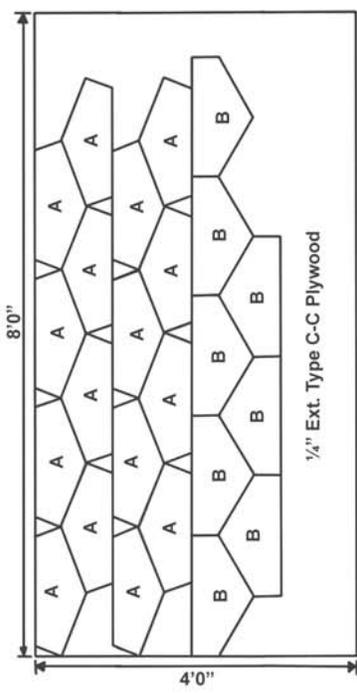
PLYWOOD SHEET CUTTING DIAGRAM
